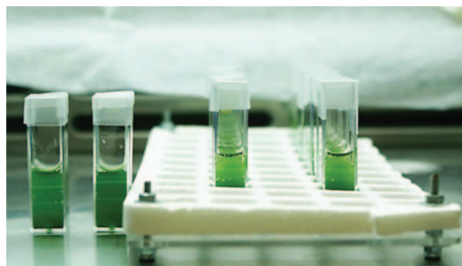
Fig. 8. High-throughput experimental design. Four clear-side cuvettes with 2 ml of Synechocystis sp. PCC 6803 culture on acrylic rack inside growth chamber (for details, see Experimental Procedures).
